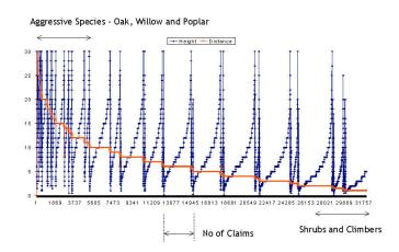
The regular signature across differing height ranges illustrates the point that the average tree poses a threat to a property wherever it is situated within a radius equal to, or less than, the tree height.
